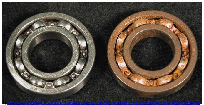
material and the conditions at the time. Commonly used are solvent cleaning, chemical cleaning and mechanical cleaning.
